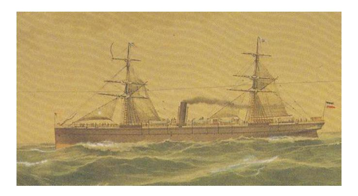
The "Vandalia" (shown here) was built in 1871 by Caird & Co, Greenock for the Hamburg-America Line. She was a 2,810 gross ton ship, length 330ft x beam 39ft, one funnel, two masts (rigged for sail), iron construction, single screw and a speed of 11 knots. There was accommodation for 150-1st, 70-2nd and 150-3rd class passengers.
